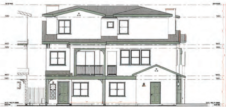
SIDE (NORTH) ELEVATION - BLDG 1 SCALE: 3/16" = 1'-0"
