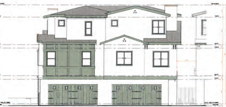
SIDE (SOUTH) ELEVATION - BLDG 1 SCALE: 3/16" = 1'-0"
