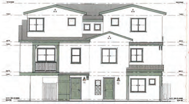
SIDE (NORTH) ELEVATION - BLDG 4 SCALE: 3/16" = 1'-0"
